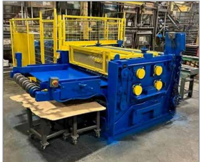
5S Project - restoration of the grain bin sidewall curving machine
